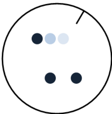
Figure 4: Symbolic illustration of a developed well with well marking for rotation correction (1 o'clock position / 30°)
